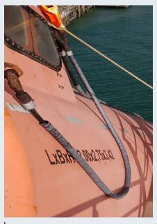
Figure 4. Alternative sheathing arrangement which allows for inspection
