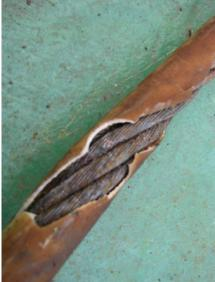
Figure 2. Corrosion beneath plastic sheathing.
