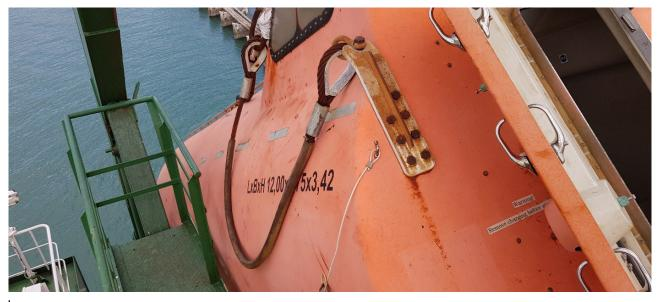
Figure 1. Lifing sling encased in plastic sheathing
