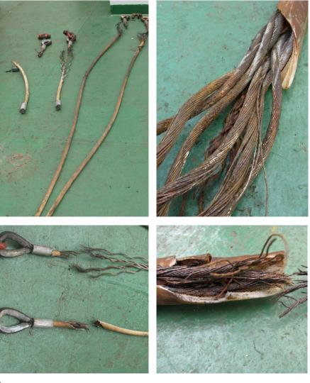
Figure 3. Lifting slings parted due to undetected corrosion.
